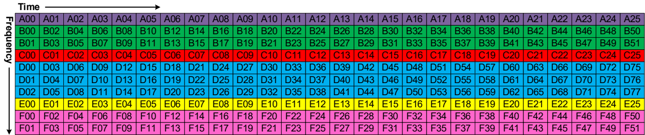
Figure 7.24 Example of frequency division multiplexing of PLPs.
